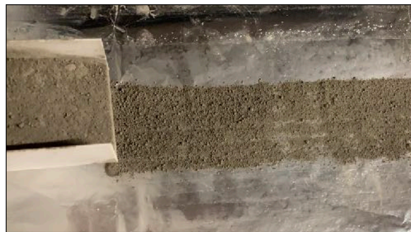
Fig. 5 - Vibration intensity + travel speed can create uniform powder beds for sintering. One without the other creates irregularities in powder bed depth.
