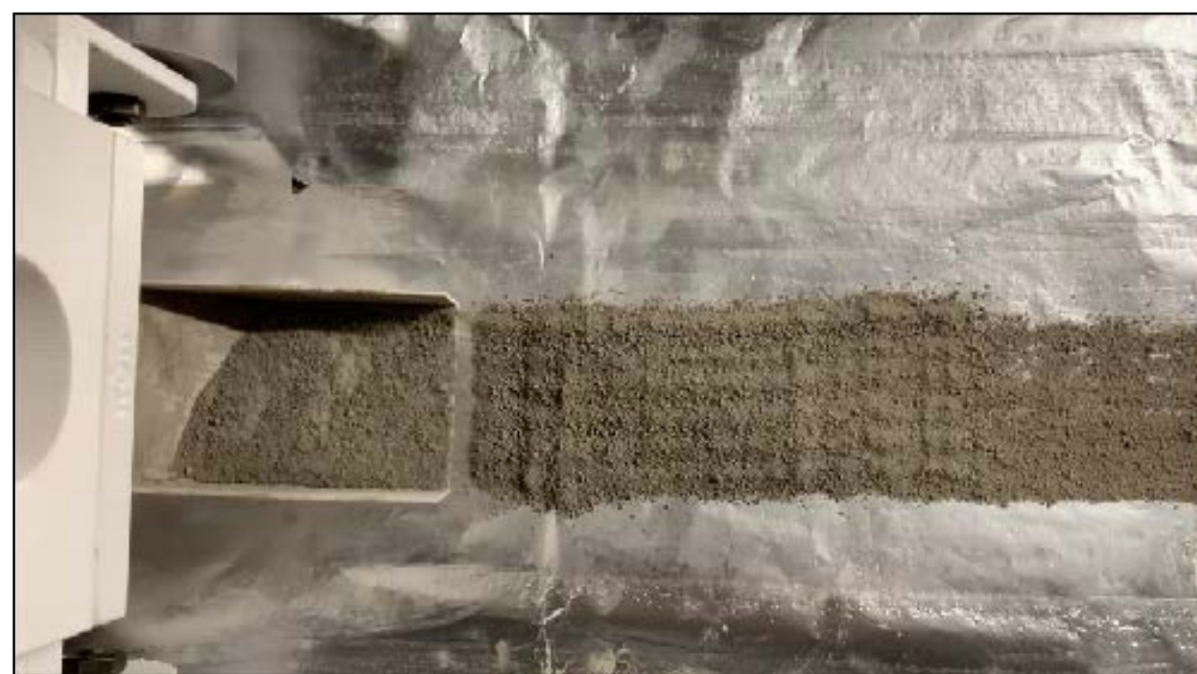
Fig. 4 - Guide vanes can leave “grooves” in powder at incorrect vibration frequencies and travel speeds
