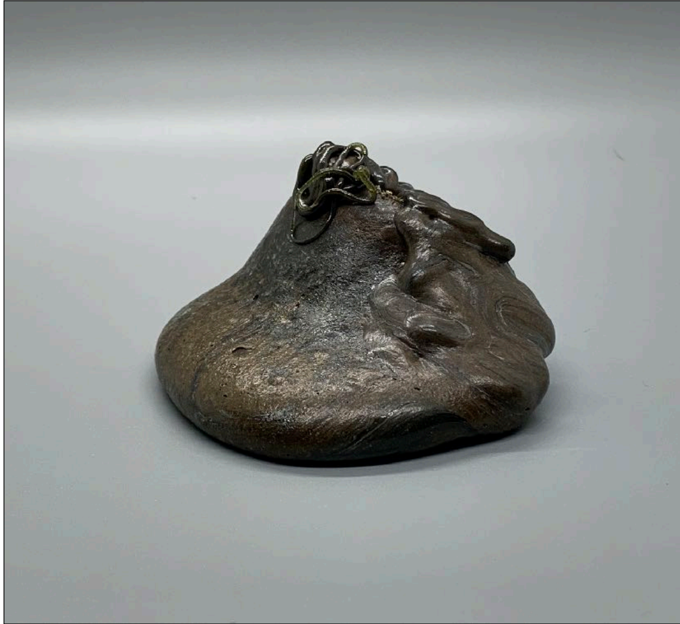
Fig. 1 - Sample 2A-006 First flowing sample of molten LHS-1 in the ICON labs.
