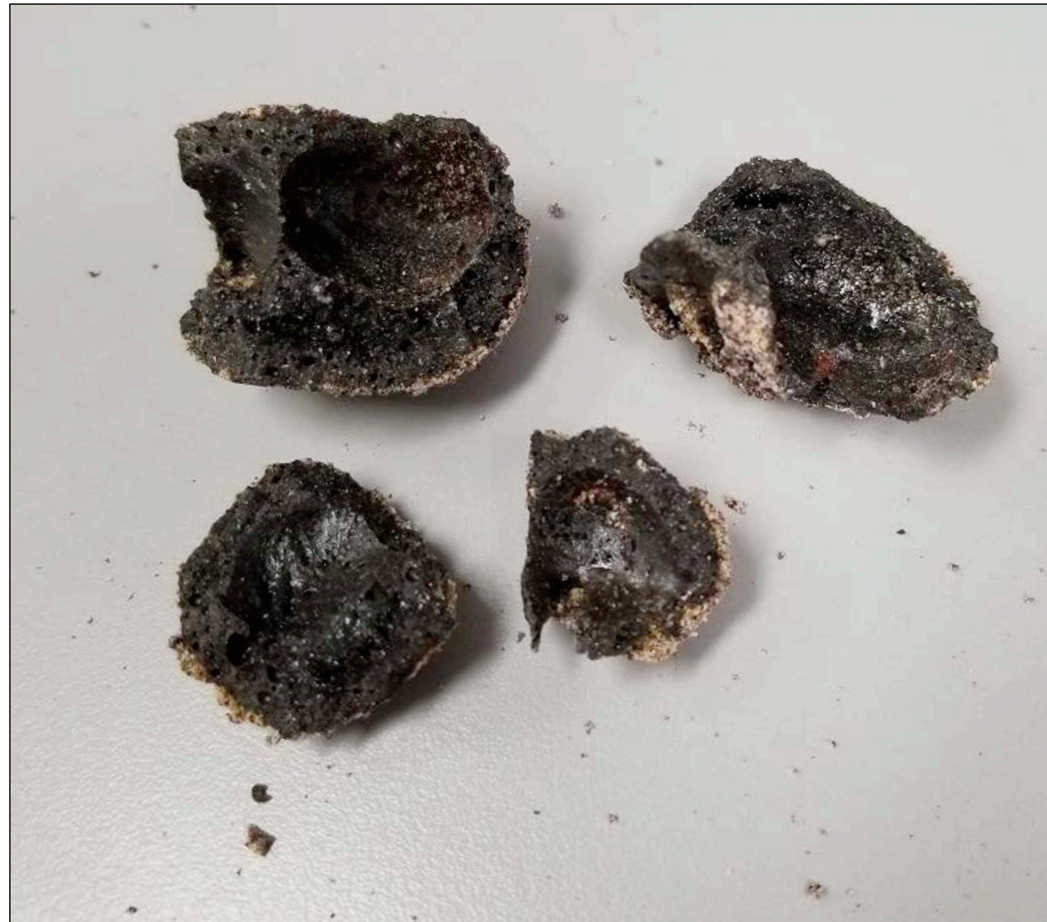
Fig. 2 - Sintered samples from test run #19 fractured for inspection
