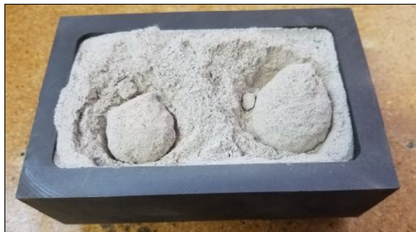
Fig. 4 - LHS-1 sample post heating from test run #15. The two areas of focused microwaves generated hot spots that sintered the regolith.
