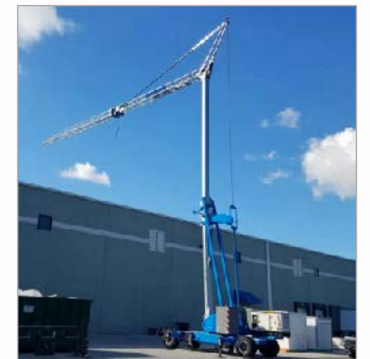
Fig. 3 - Self-Propelled, Self-Erecting Tower Crane found in smaller scale construction applications on Earth
