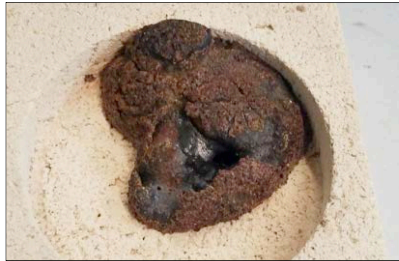
Fig. 2 - Test run #7, LHS-1 heating in refractory brick crucible, Refractory bricks can be sintered to LHS-1 is the hotspot is hot enough.
