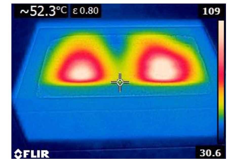
Fig. 4 - ICON successfully demonstrated that changing microwave frequency moves the hot spot in the multimode cavity to heat and sinter new material. This IR imagery shows a LHS-1 sample heating in a graphite crucible from test run #15.
