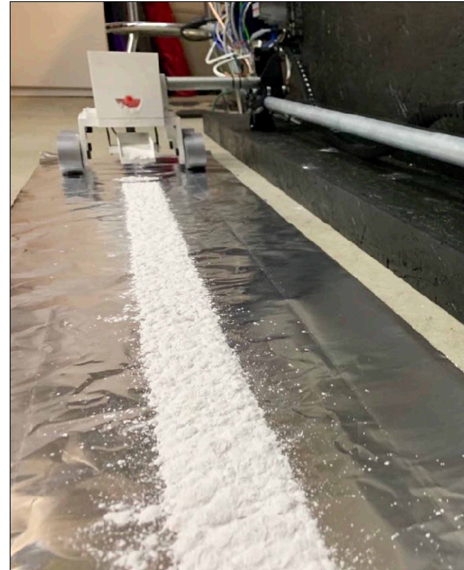
Fig. 2 - BB-04 deposition experiments using Greenspar 90 material for calibration
