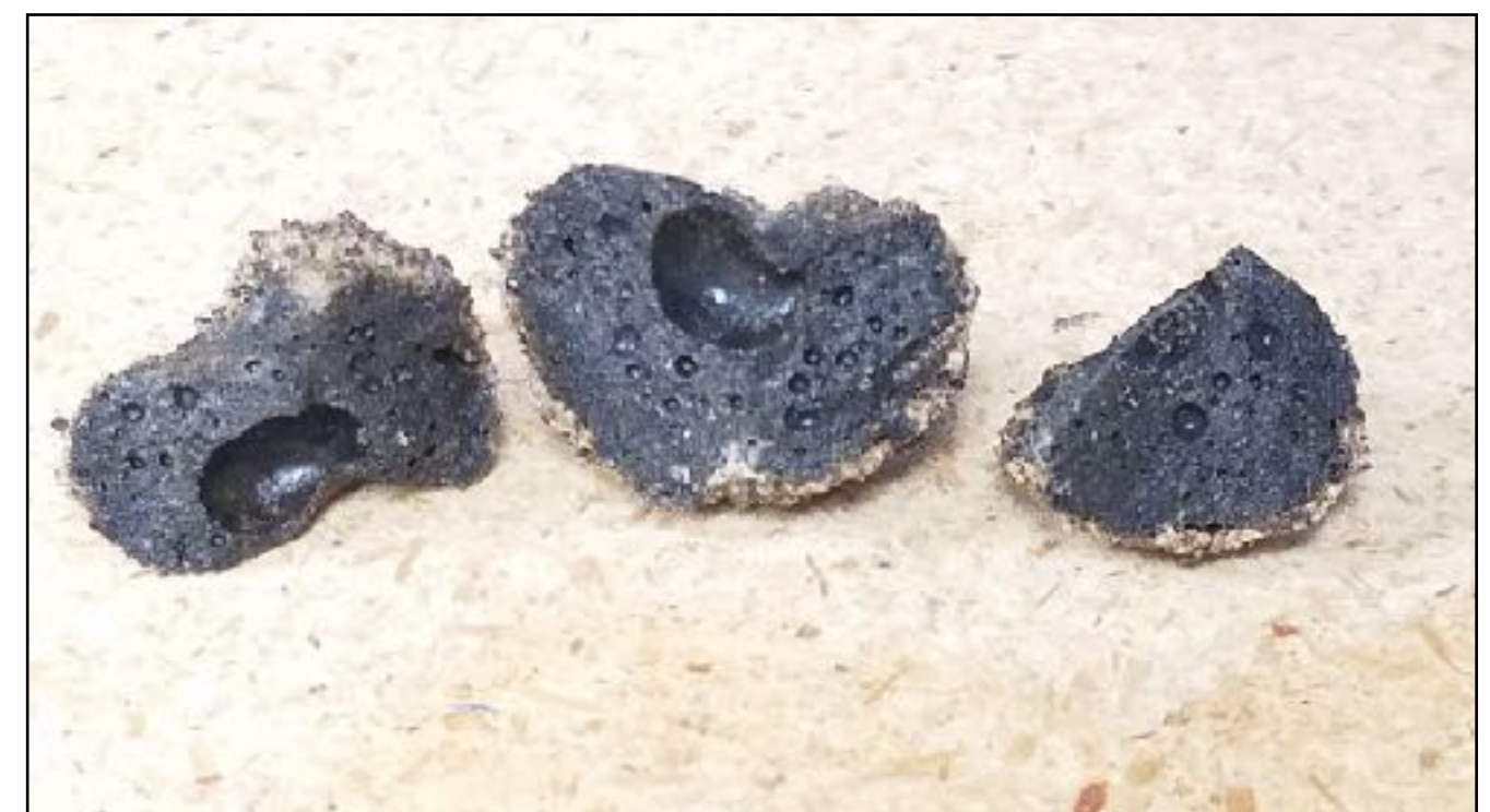
Fig. 6 - LHS-1 sample broken open from test run #15. Voiding appears to be caused by off-gassing of regolith during the heating process.
