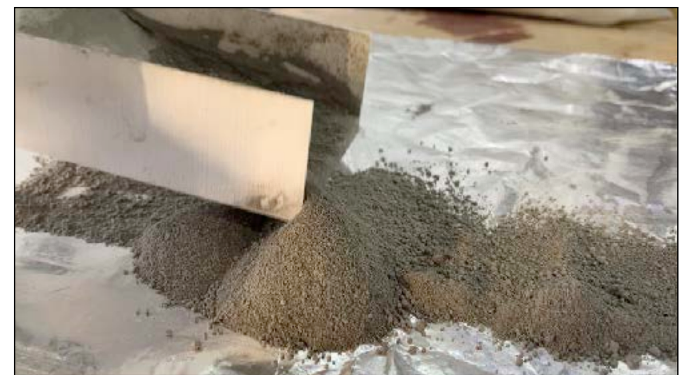
Fig. 6 - Centripetal force from the vibration motor's axis being aligned with the vibration plate's center line allows regolith to be moved from left / right inside the vibration plate dependent on motor direction. Pulsing the vibration motor and/or reversing motor direction provide for “cleaning” of the vibration plate.
